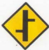
Junction ahead with road or roads of less importance (indicated by arms of lesser width)
